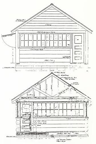
Figure 59. Log lookout house, Plan L-5, designed in 1928 for the Northern District. Roughly 18 feet by 14 feet, it provided both living and working space for the lookout. Its windows, with up to 30 panes to a side, provided good views.
